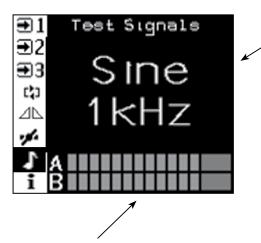
Loop Current bar graph for each channel. Shows Loop output current in 2dB steps from >-20dB to 0dB in green. Red = clipping Test signal selected by rotary control:
