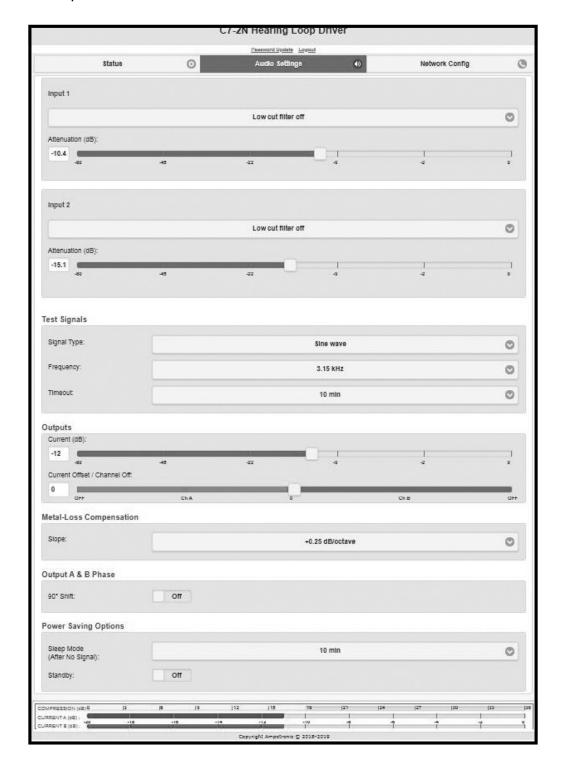
The title of the web page is always CX-XX where Xs are dependent on the driver type. At the bottom of the screen are the meters for the level of compression and the current in loop A (and B if present).
